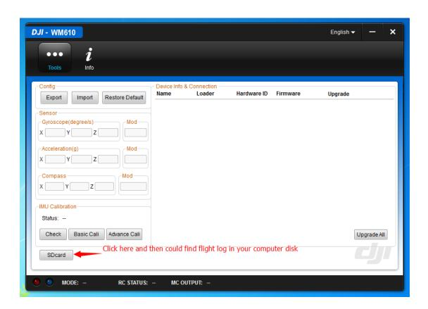
Step3: Then you would find a disk named as "DJI FLY LOG", you could find related log in this disk. Please send the corresponding log to us with specific description.
